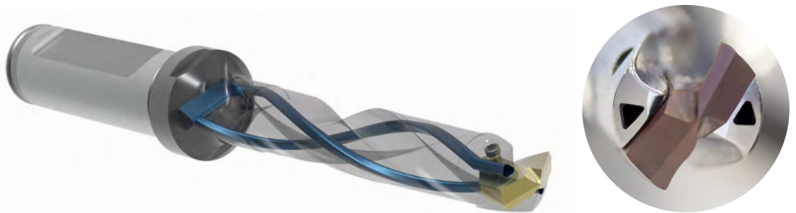
Fig. 6: Indexable insert drill QTD from MAPAL with non-circular cooling channel profile to increase the coolant flow and spiral cooling channels.
