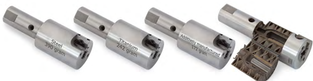
Fig. 7: Mass reduction on a MAPAL external reamer from 390 g to 172 g due to a specially developed ribbed structure inside the tool.
